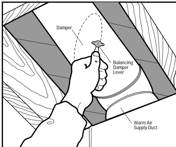
In some forced-air distribution systems, balancing dampers may be located in the secondary warm air ducts, close to where they branch off from the rectangular main heating duct. Often the dampers can be identified by a small lever on the outside of the duct (Figure 5). The position of this lever (or sometimes a slot in the end of the damper shaft) indicates the angle of the unseen damper inside the duct. If there are no such dampers, you will have to use the ones in the floor registers.
