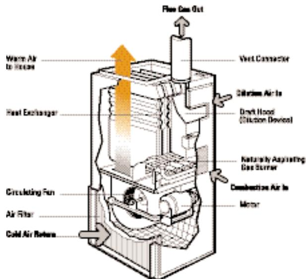
by pulling varying quantities of heated house air into the exhaust as required. A circulating fan passes cooled house air from the return ducts over the furnace heat exchanger, where the air is warmed up and passed into the ductwork that distributes the heated air around the house.
