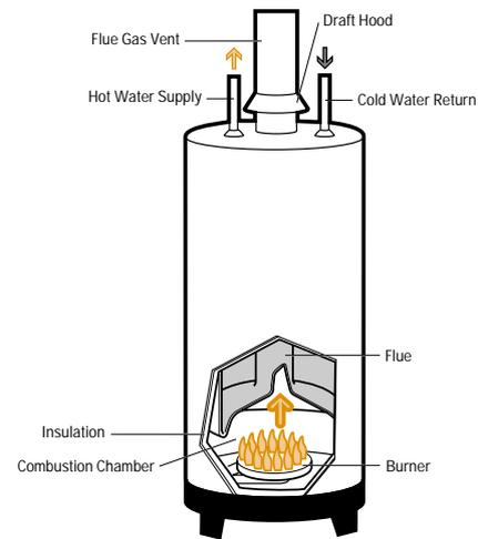
A combined combustion thermostat and gas valve unit controls both the temperature of the water in the tank and the gas flow. The flue passes vertically through the centre of the tank cylinder to the outside. Its main job is to conduct the combustion products from the combustion chamber to the vent system. Approximately one-half to two-thirds of the standby losses are through the flue. Overall seasonal efficiencies are around 55 to 60 percent.
