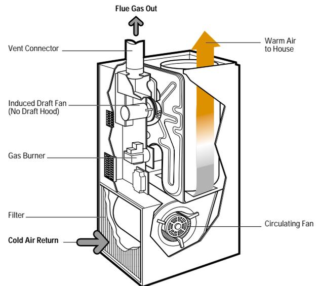
Note that installation codes may require a combustion air supply to be brought from outdoors to the furnace.
